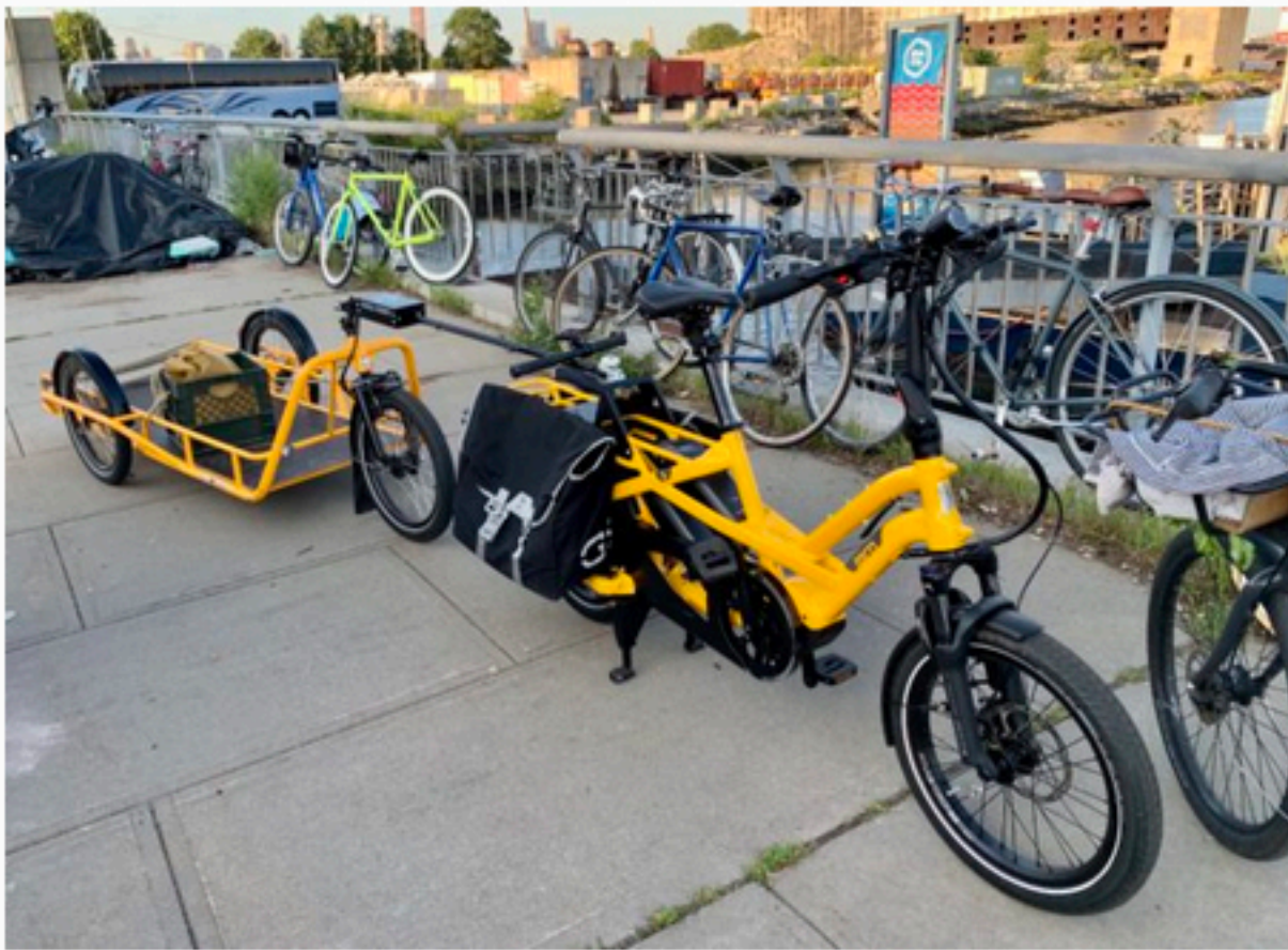
Solar-powered cargo bikes used to deliver cargo the last mile. Photo: Mary Frost/Brooklyn Eagle
