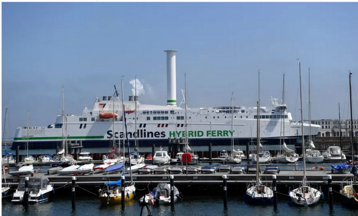
A Flettner rotor on a Danish hybrid ferry in 2020. Photograph: Annegret Hilse/Reuters
